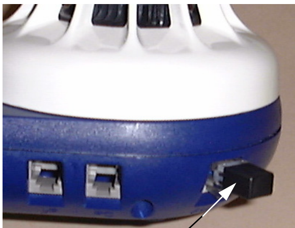
Ex Dongle Adaptor fitted to 801AP 'AUX' port
