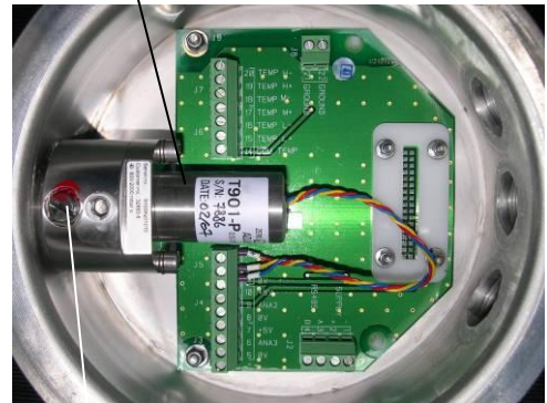
Isolating valve of the pressure sensor
